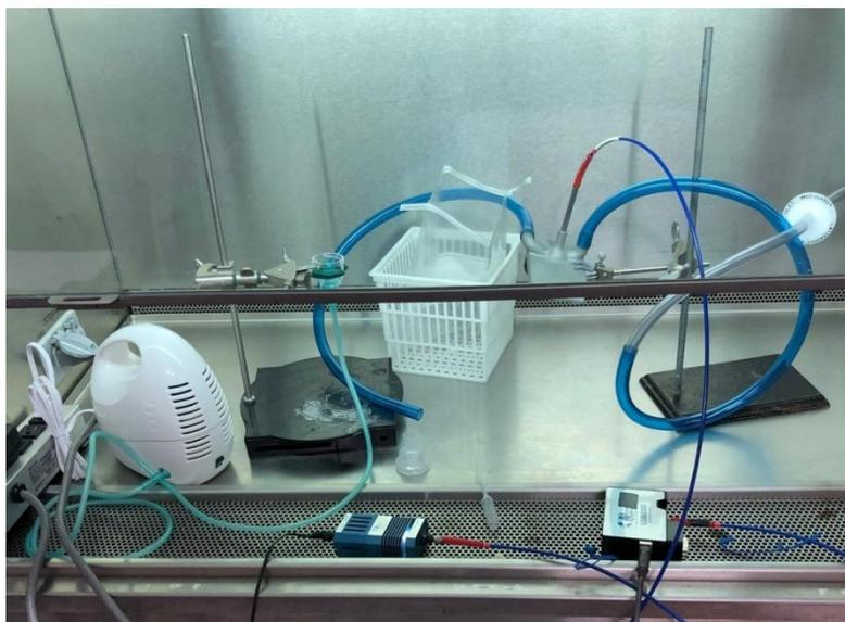
Figure 1. Biosensor developed by Phoenix Biometrics Inc. The water sample was introduced by the nebulizer to the biofilm chamber and detected by the light probe.
