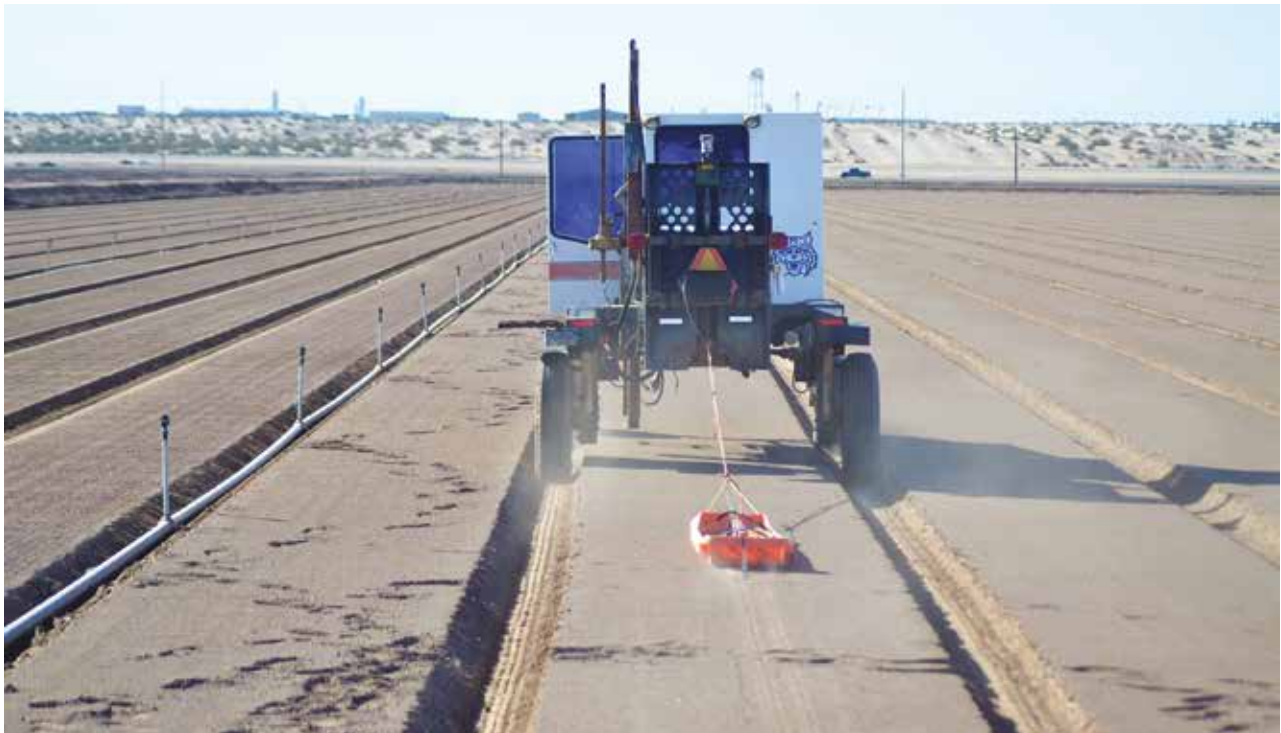
Figure 7. EM38 pre-plant conductance survey.
